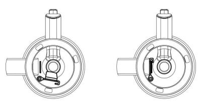
assemble bowl onto the base. Put bowl on the base and clockwise rotate to lock the blow.
