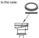
7.Put the filter case back to the dust cup 8. Assemble the dust cup to the mainbody.
