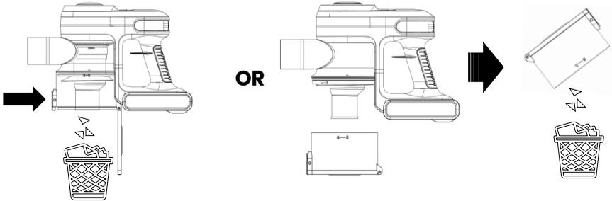
2. Lift out the filter mask by twisting count clockwise and pulling it out.
