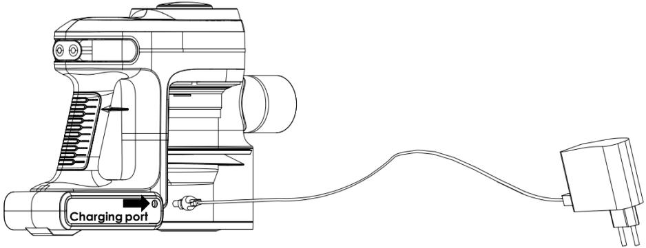
Plug the adapter into the charging port and then plug the other side of the adapter into the power outlet.
